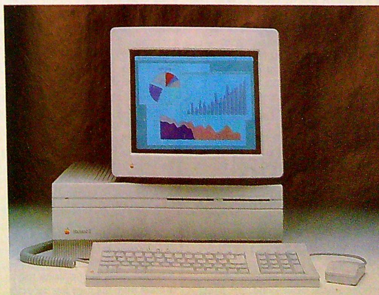
The Macintosh II looks nothing like a Macintosh. Its separate system unit and display make it appear similar to the Apple IIgs. This Mac II is equipped with the optional color display.
